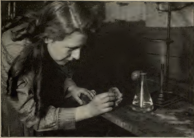
FIG. 52. A toy balloon has been slipped over the mouth of a flask that is filled with steam.
